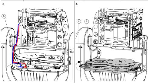
To remove the Colors and Fixed Gobo wheels module:
