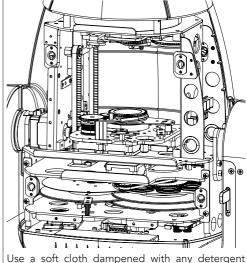
Before removing rear cover, place the head in a horizontal position and engage both the PAN and TILT locks for added stability. See the "PAN | from the reflectors, from the lenses and filters. AND TILT LOCK" paragrap (pag. 6). Loosen and remove the marked screws and opening the head covers (1) from both sides.
