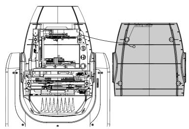
Unclip the safety cable on both sides (2).
