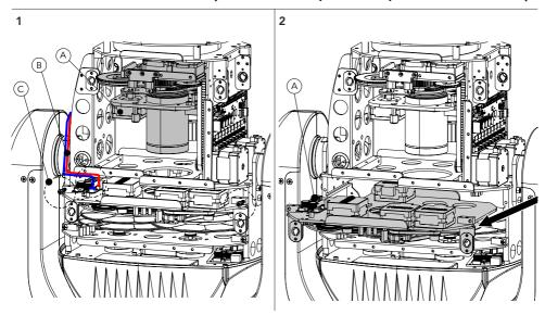
To remove the Animation and Gobo wheels module, open the head covers (see section "PERIODIC CLEANING") and proceed as follows:
